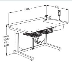
**Height-adjustable** from 650 – 1000 mm **Max. load R8652, R8654:** 75 kg
