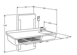
Height-adjustable from 300 – 1000 mm Max. load R8782 - R8785: 75 kg
