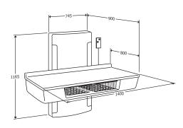
Height-adjustable from 300 – 1000 mm Max. load R8762 - R8763: 75 kg
